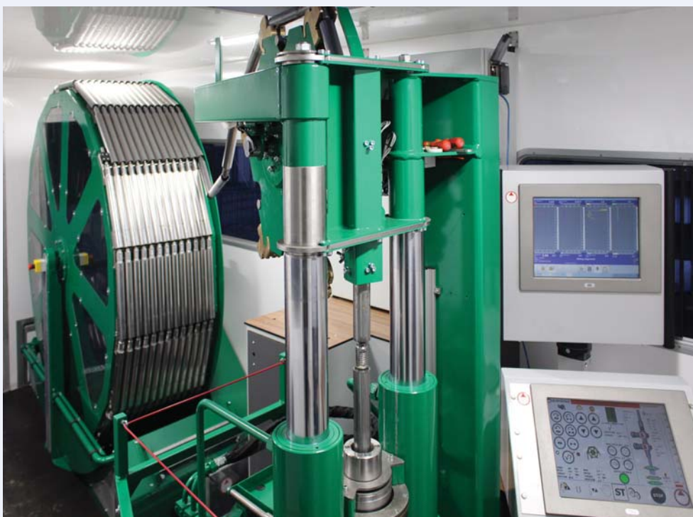
Figure 1 – Automatic and hands-free CPT machine.
