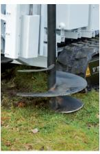
The Midi CPT Crawler consists of our proven HYSON 200 kN pene-trometer mounted on an undercar-riage with rubber tracks. The Midi CPT Crawler from A.P. van den Berg is designed to be compact, manoeuvrable and light, but with maximum power. With a weight of about 3,500 kilo and a width of only 1,200 mm the Midi CPT Craw-ler fits trough small passages and can be transported in a small truck. All these features ensure that the
