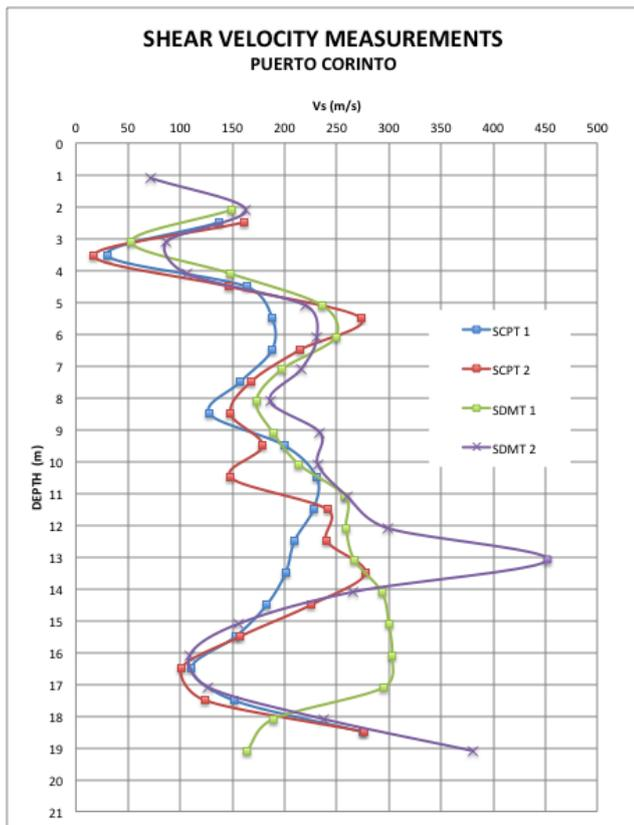
Fig. 16. Comparison of the shear velocity between two different sets of equipment.
