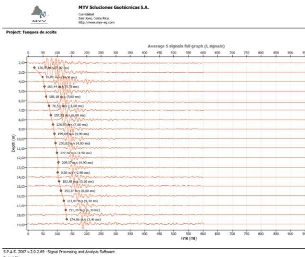
Fig. 15. Data output of the Seismic module. Given that 2 seismic dilatometer and 2 seismic CPTs were carried out, a comparison among the different shear velocity profiles was possible.
