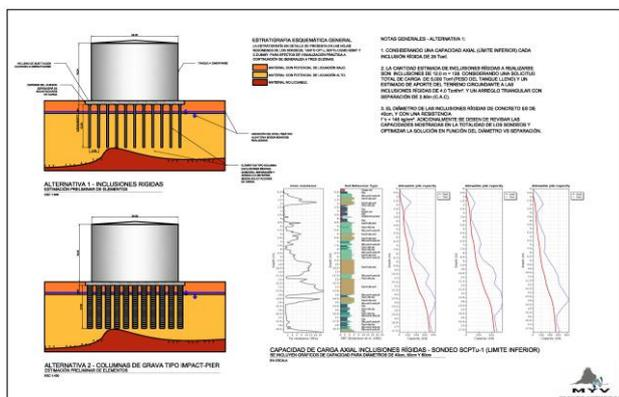
Fig. 14. Proposed foundation for the tank.
