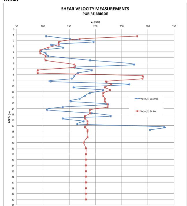
Fig. 13. Comparison between  $V_s$  from SCPTu and  $V_s$  from SASW.
