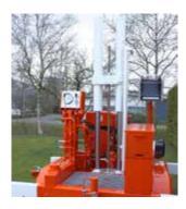
**CPT Trailer versus large self-propelled machines** The 20 tons CPT Trailer provides the same high penetration force as the CPT truck, Track-Truck and CPT Crawler, but at significantly lower capital cost. The main difference between the trailer versus the large self-propelled machines is that those carry their own ballast weight; whereas
