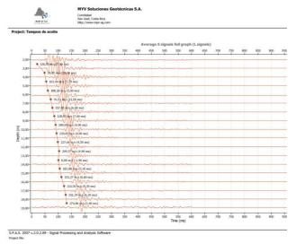
Fig. 15. Data output of the Seismic module. Given that 2 seismic dilatometer and 2 seismic CPTs were carried out, a comparison among the different shear velocity profiles was possible. The results of this comparison are shown in figure 16.
