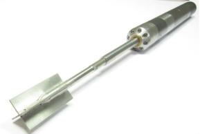
Fig. 10. Icone vane (without protection tube).
