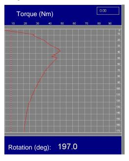
Fig. 11. Results of an Icone vane test.
