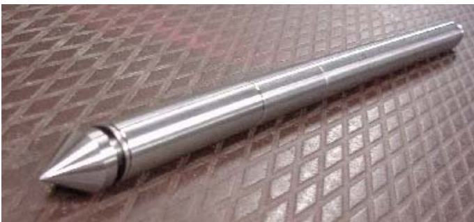
Figure 5: 2.6 cm 2 cone, depth rated 4000 m.
