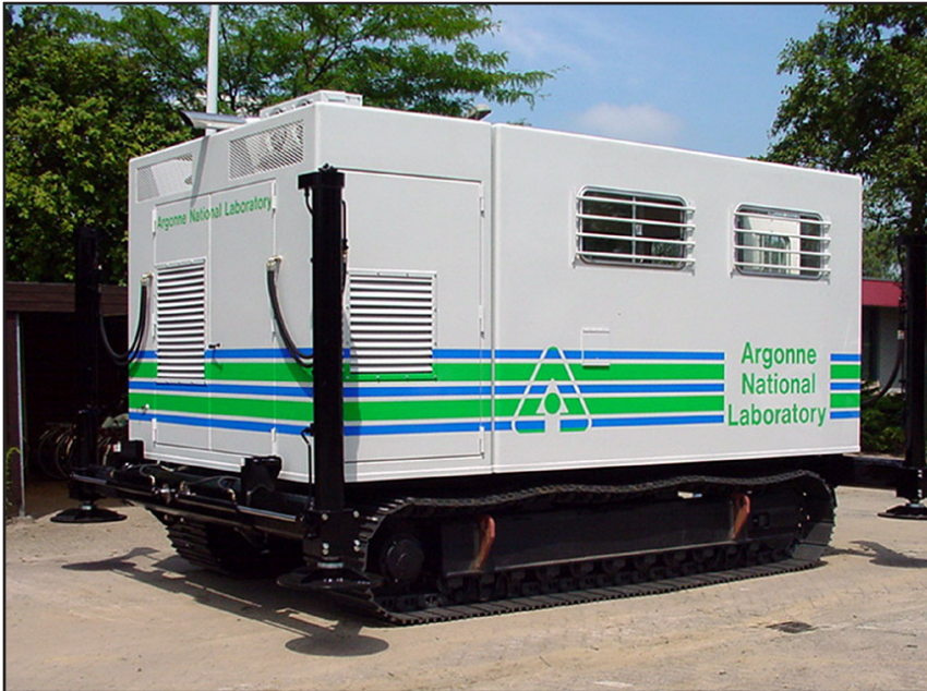
Argonne uses the direct-push capabilities of this cone penetrometer vehicle to explore the subsurface environment.
